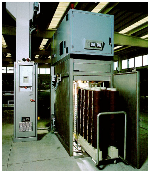
Fig. 2: 60 kW with single carrier for yarn packages capacity 100-120 kgs/batch
